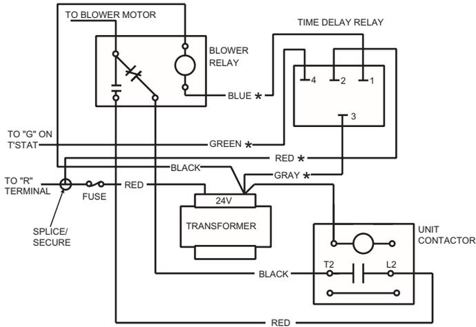
\* WIRES MARKED WITH AN ASTERISK (\*) ARE SUPPLIED AS PART OF TDR KIT.
