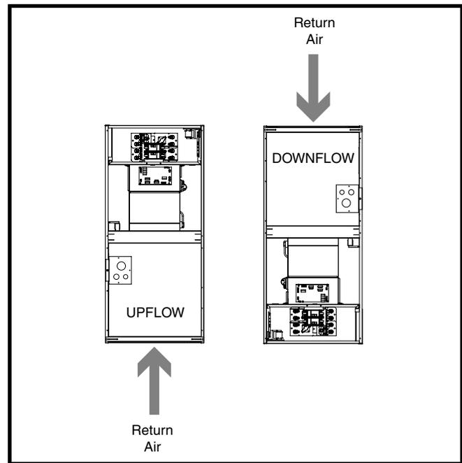
**Figure 2. Installation Configurations**
