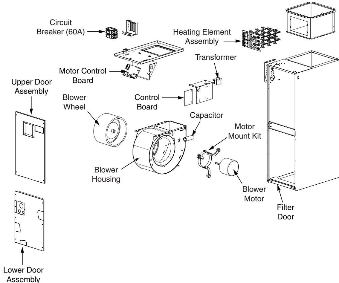
Figure 7. B6BV Series Air Handler Components
