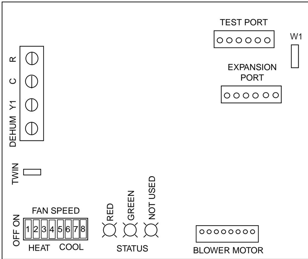
Figure 12. Two-Stage Fixed Speed Motor Control Board (MB7EM Models)
