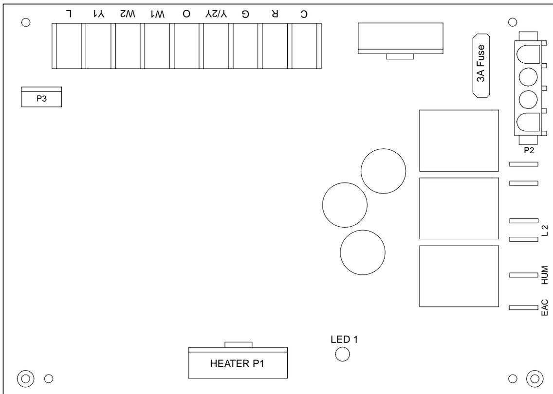
**Figure 11. Two - Stage Control Board (MB7EM / VM Models)**
