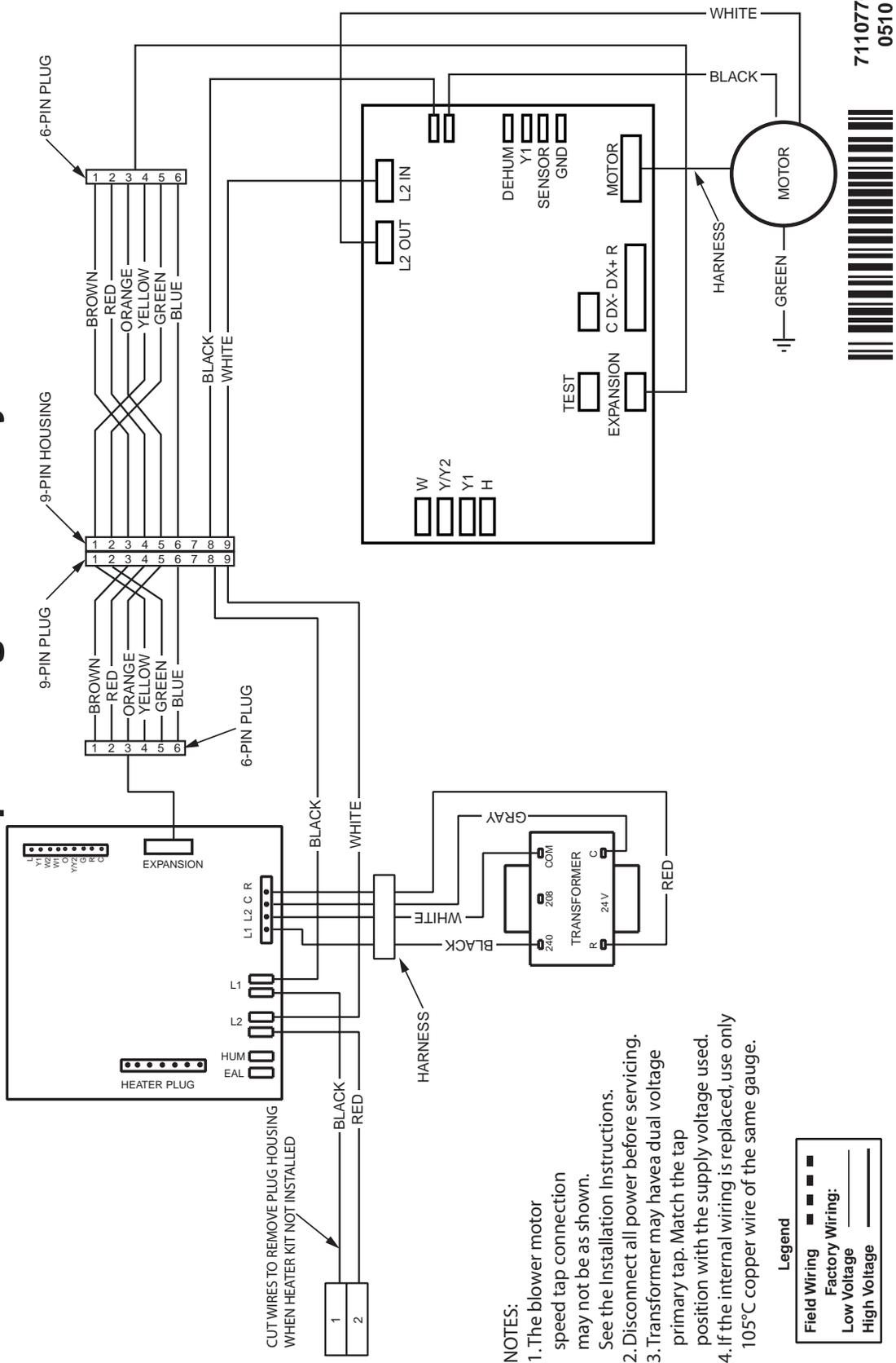
Figure 16. Wiring Diagram for MB7VM Series Air Handler
