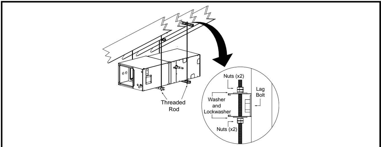
Figure 5. Unit Horizontally Suspended
