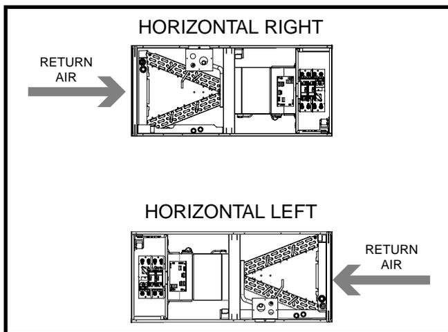
Figure 3. Horizontal Configurations
