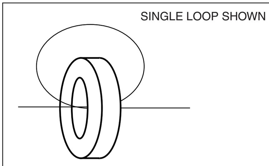
**Figure 3. Noise Reduction Toroid**
