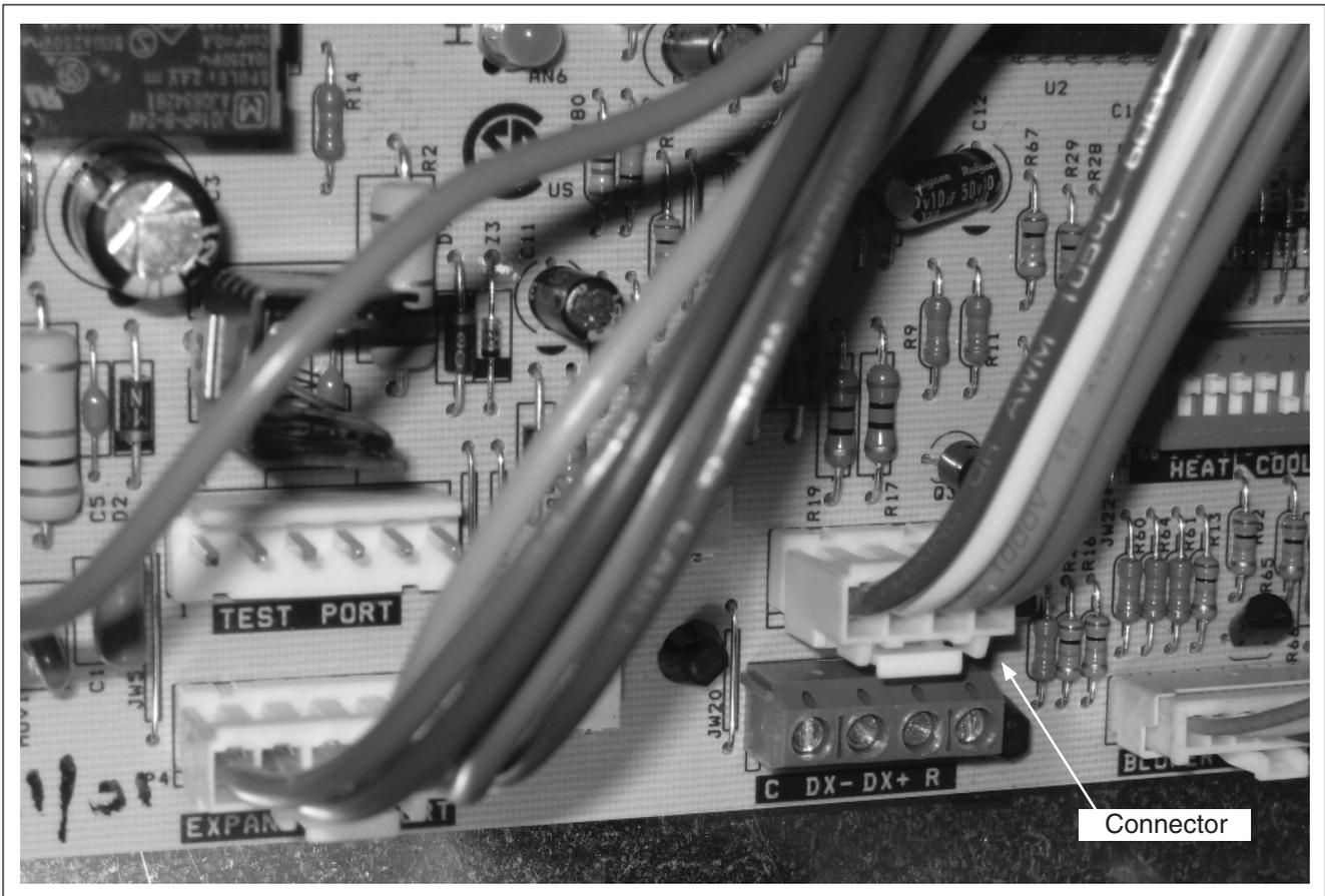
Figure 16. Four-wire connector on Motor Control Board
