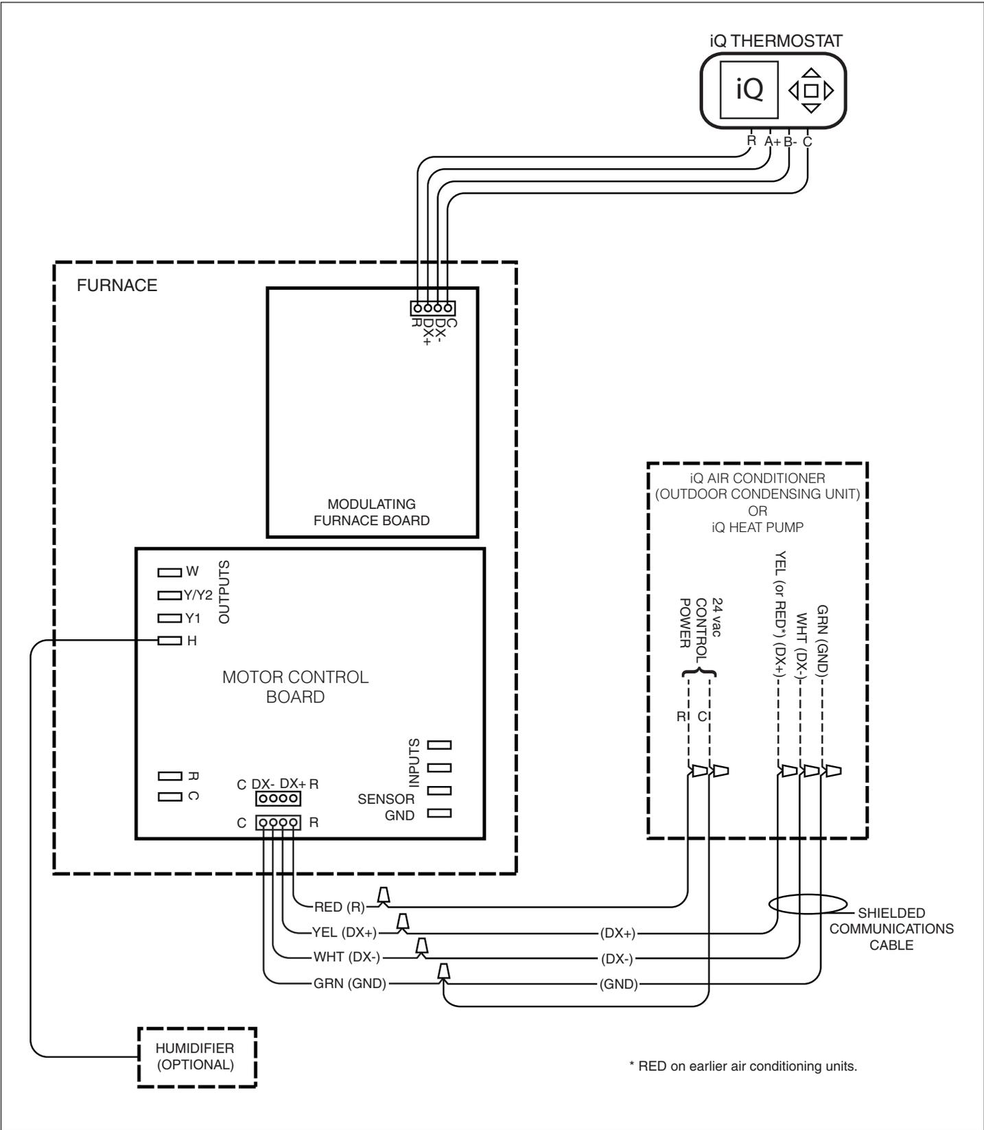
Figure 22. Control Wire Connections, G7 Modulating Gas Furnace
