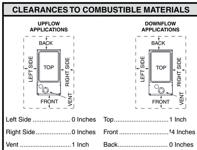
\*Allow 24 in. minimum clearance for servicing. Recommended clearance is 36 in.
