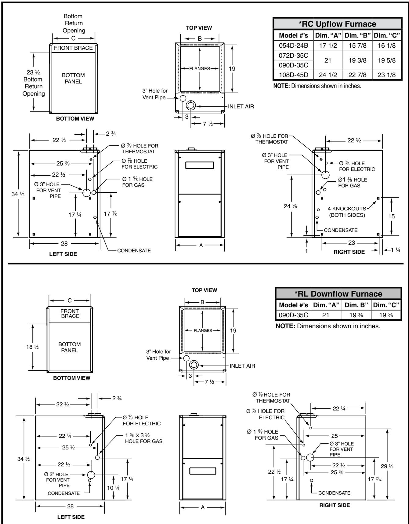
**Figure 41. Furnace Dimensions**
