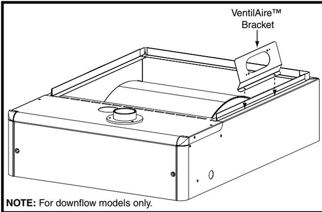
**Figure 33. VentilAire™ Bracket**
