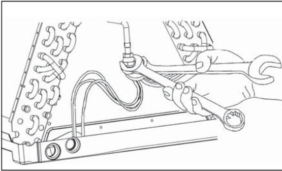
**Figure 5. Wrenches on Distributor Body and Assembly Nut**
