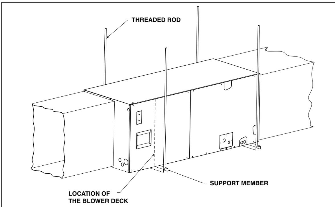
**Figure 4. Typical Horizontal Installation Using Threaded Rod and Supporting Members (Shown in Horizontal Left Position)**
