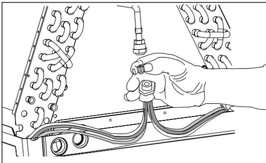
**Figure 7. Orifice Insertion in Distributor Body**
