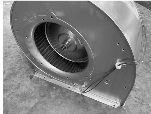
Figure 8. Blower Limit Switches/Wires
