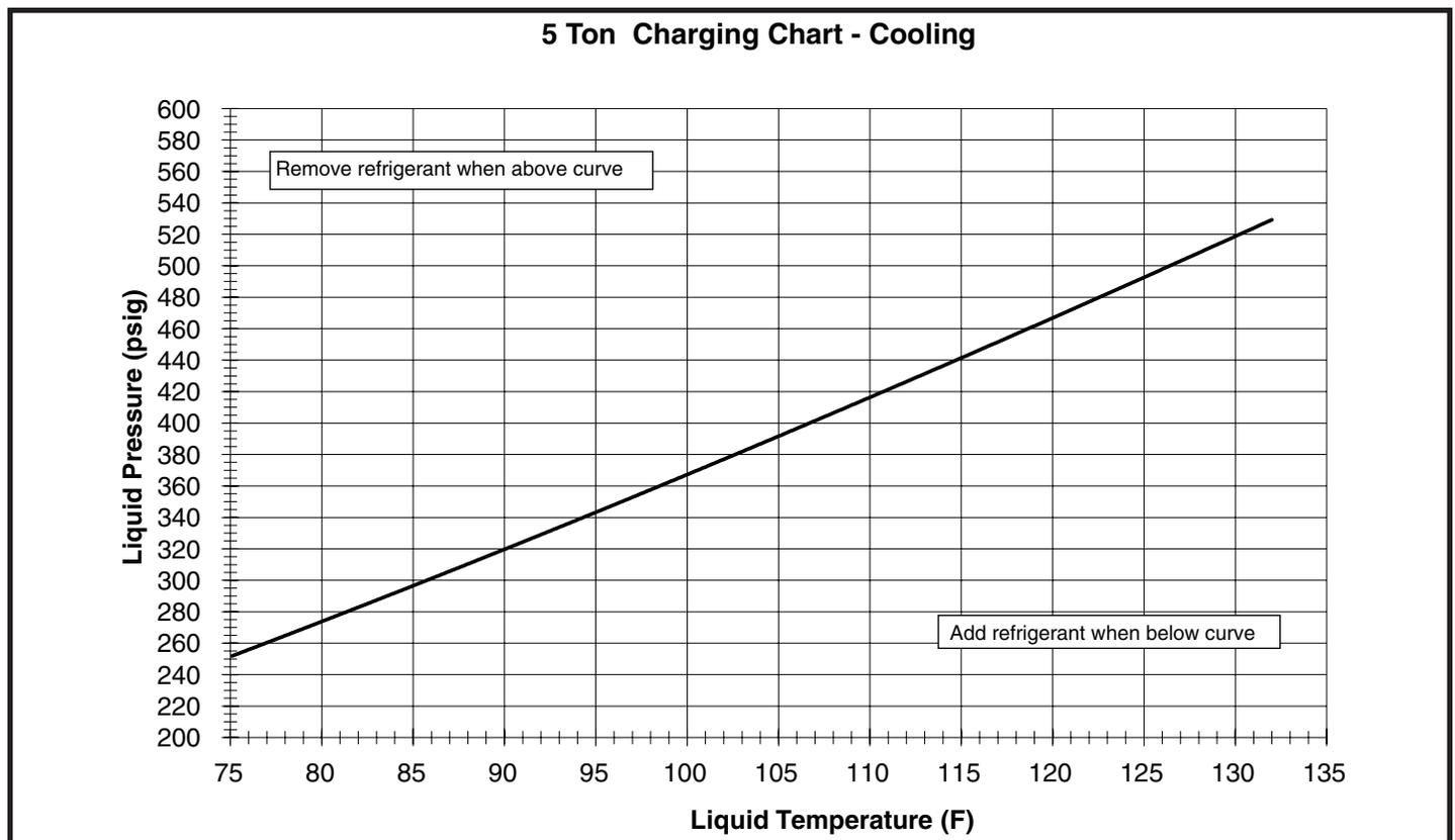
Figure 13. Charging Chart for 5 Ton Models
