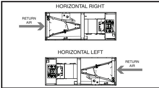
**Figure 3. Horizontal Configurations**
