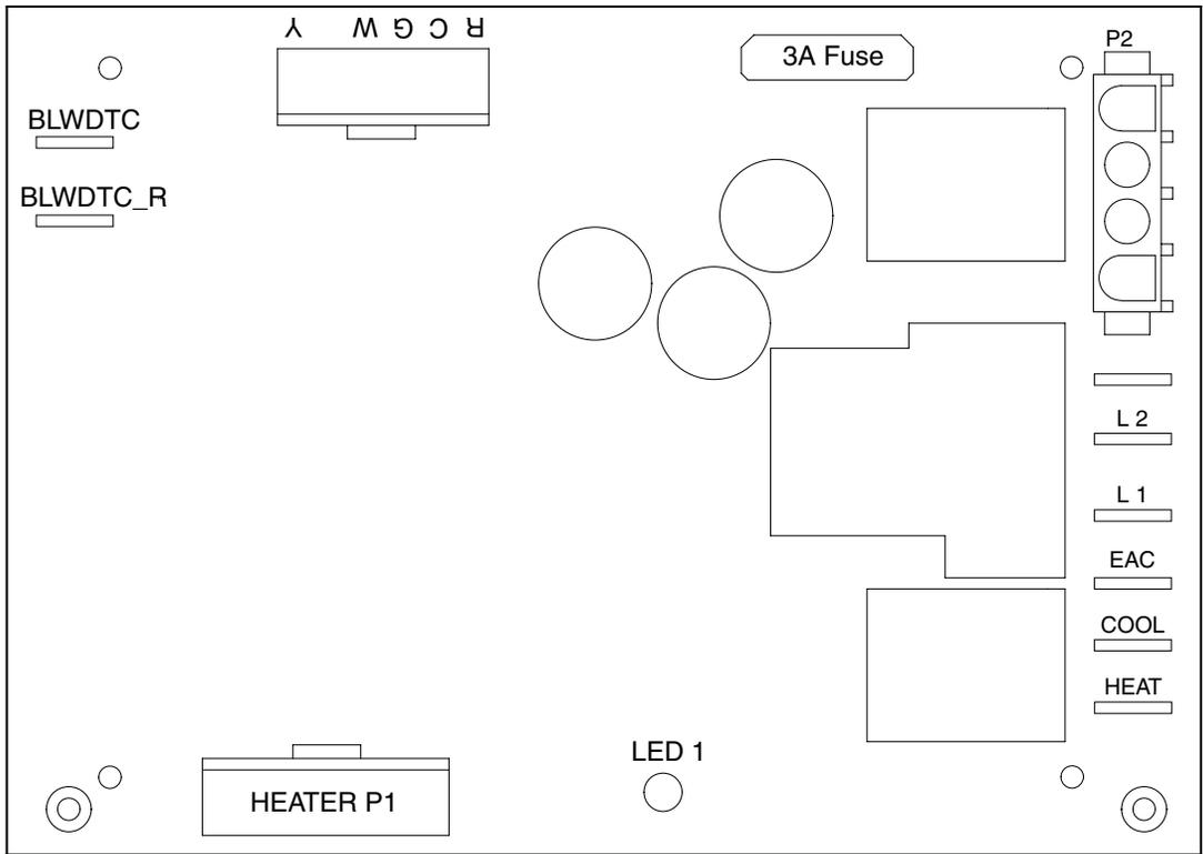
Figure 15. Single Stage Control Board
