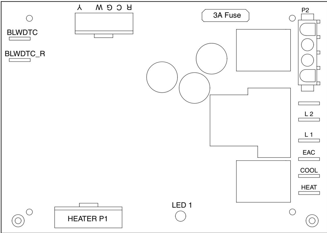
Figure 11. Single Stage Control Board (MB7BM Models)
