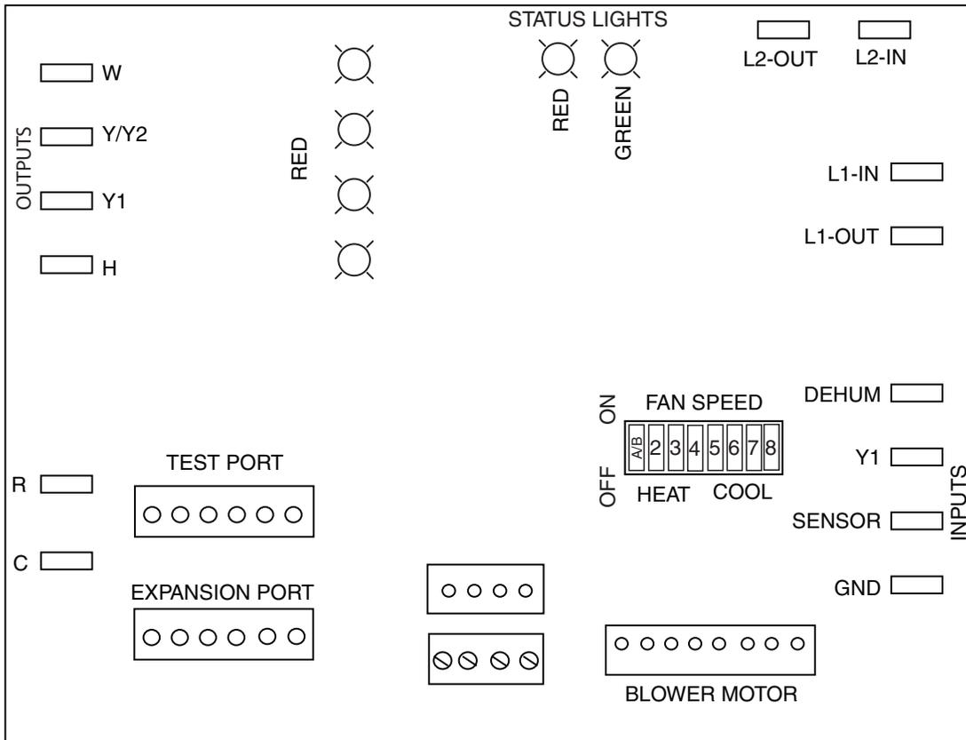
Figure 14. Variable Speed Motor Control Board (MB7VM Models)
